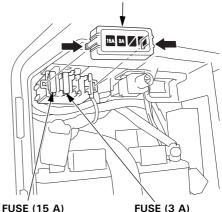
5. Install the fuse holder cover and the battery maintenance cover in the reverse order of removal (see page 51). Never operate the generator with the battery maintenance cover open, as poor engine and generator performance will result.
