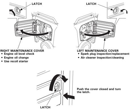
Be sure the maintenance covers are closed while the generator is running.
