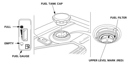
After refueling, reinstall the fuel tank cap securely.
